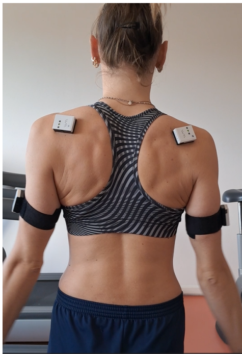
Figure 1: The adopted measuring protocol is visible in the photo. Two sensors are on each shoulder, two on the humerus and 1 (not visible) on the thorax.
