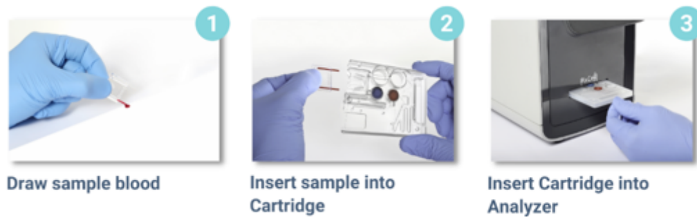
Figure 1: 1. Filling the capillaries with blood. 2. Inserting the capillaries into the cartridge. 3. Placing the cartridge into the analyzer.
