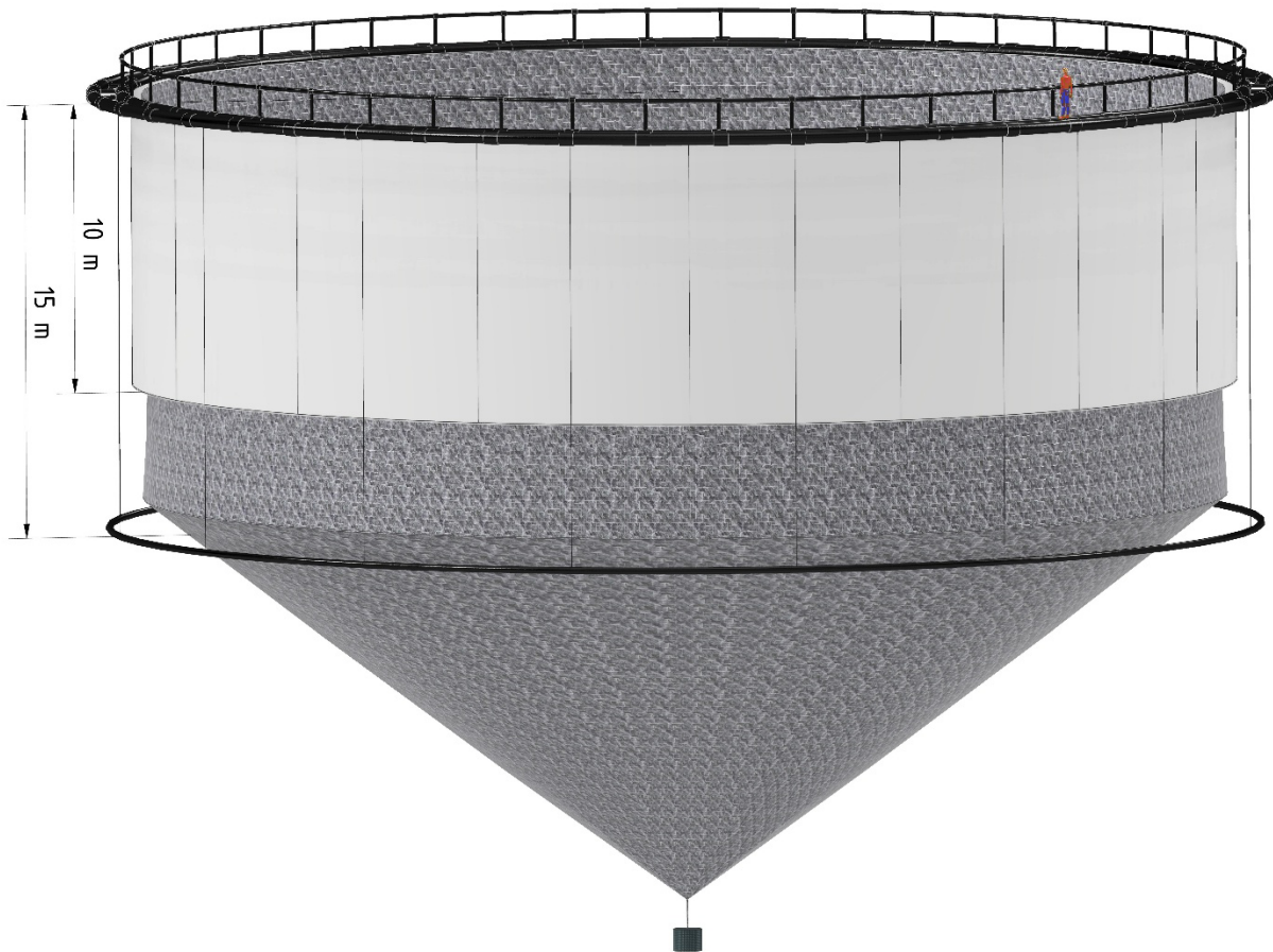
Figure 2: A 10 m deep lice-shielding skirt in a circular 120 m circumference cage (design: Svein B. Tveiten).
