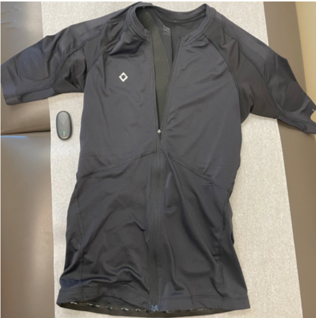
Figure 1: Athos T-shirt with surface EMG sensors embedded
