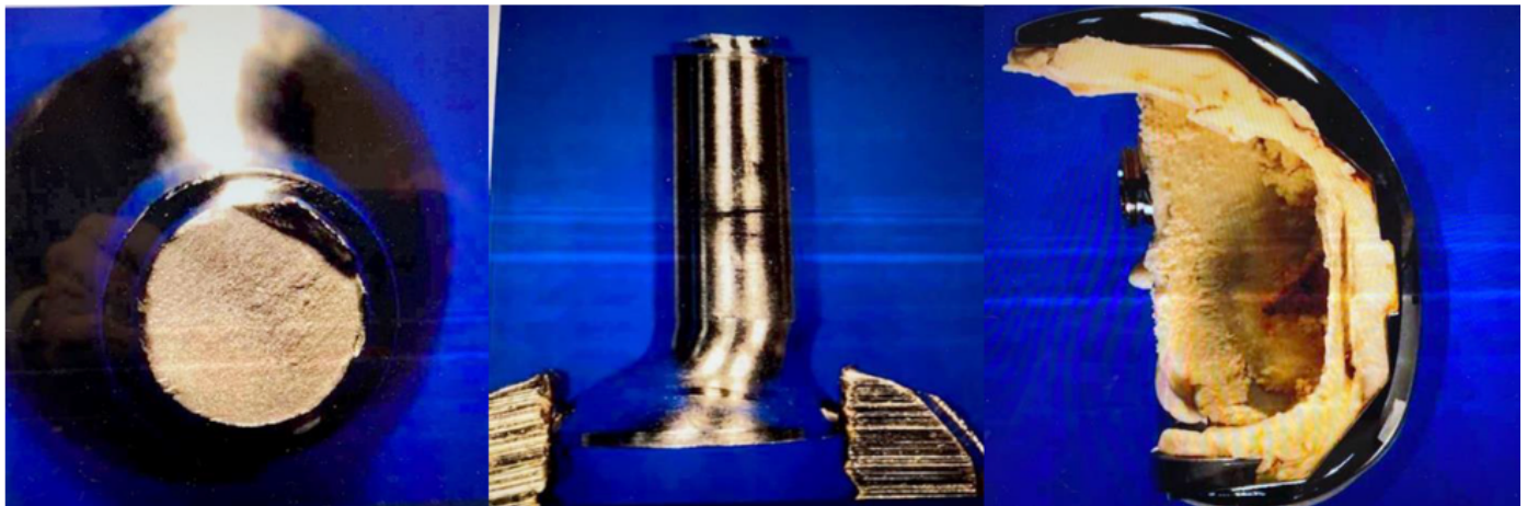
Figure 5: Broken cemented screw in the femoral component. Notice that the distal bone and cement firmly adhered to the femoral component, indicating there was no loosening but a distal fracture.
