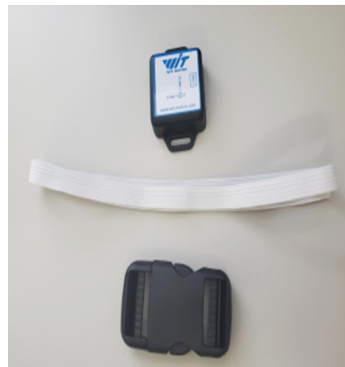
Figure 2: The WitMotion Sensor and all items needed to complete wearable function.
