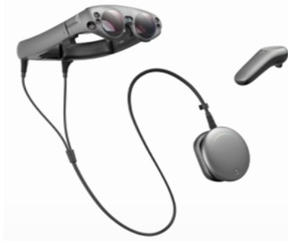
Figure 1: The ML1 device contains the lightwear (goggles), lightpack (CPU), and remote control.
