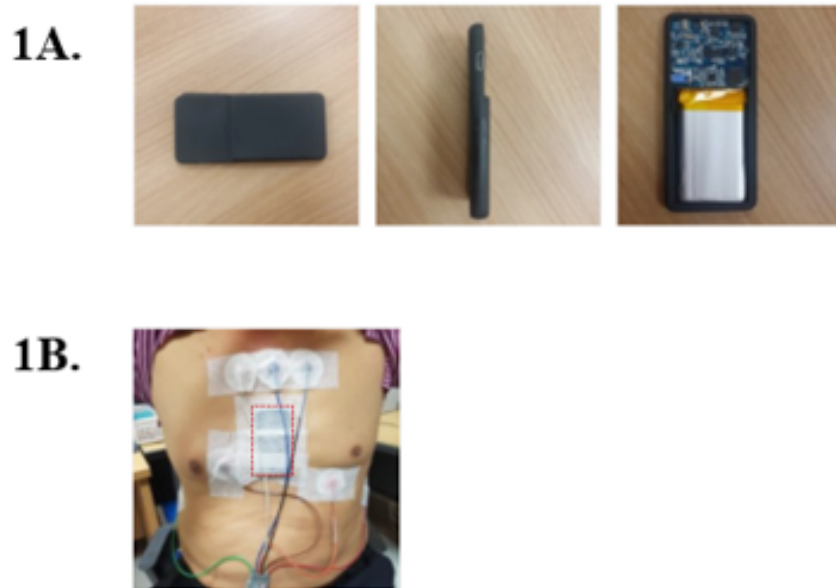
Figure 1: The inertial measurement unit-based human motion sensor: front (left), side (middle), inside (right) (A). The sensor was attached on the upper sternum (red quadrangle) simultaneously with electrodes for electrocardiogram monitoring (B).
