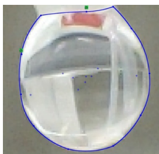
Figure 4: Magnified view of a drop with its boundary defined in a CAD software (SolidWorks 2018).
