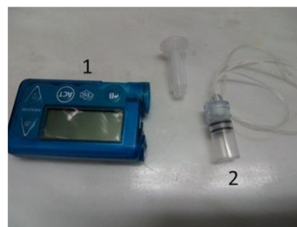
Figure 1: Equipment under calibration, where 1 is the insulin pump and 2 is the volume chamber with the capillary tube.
