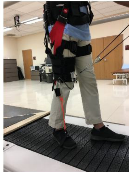
Figure 2: The assistive device used to assist the participants in hip flexion and ankle dorsiflexion at the swing phase of a gait cycle on the affected side.
