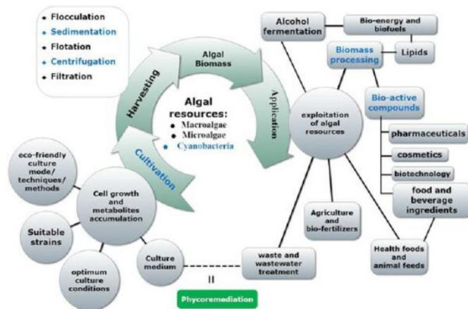
**Figure 4:** Flowsheet of algal resources production process and applications
