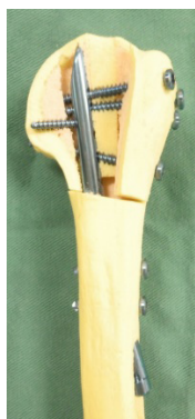
Figure 1A: The retrograde intramedullary nail in the bone model on AP view.
