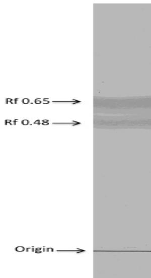
**Figure 1:** Silica gel thin layer chromatography of acid hydrolysate of dinitrophenylated LPXTGase. LPXTGase was dinitrophenylated and hydrolyzed with 6N HCl as described in methods. Running solvent was water/isopropanol/ethyl acetate (1:3:1).
