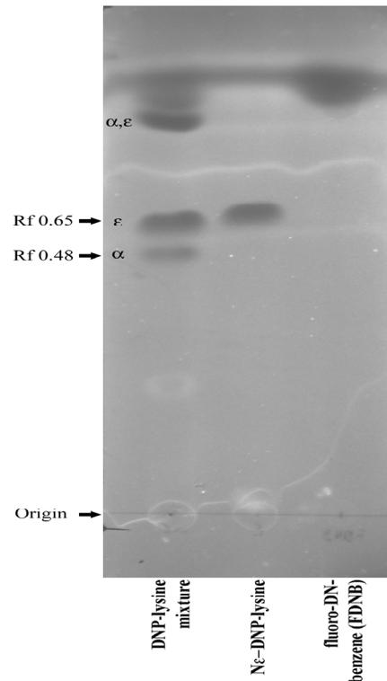
**Figure 3:** Separation of N $\alpha$ -DNP-283 lysine, N $\epsilon$ -DNP-lysine and N $\alpha$ , $\epsilon$ -di-DNP-lysine by silica gel thin layer chromatography. DNP-lysine mixture, standard N $\epsilon$ -DNP-lysine, and FDNB alone, were separated using water/isopropanol/ ethyl acetate (1:3:1) as running solvent. DNP-lysine species were prepared as described in Methods.
