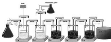
Figure 3 The schematics diagram of a simulator of the human intestinal microbial ecosystem. Source: van de Wiele et al. [14]
