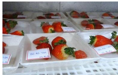
**Figure 1:** Strawberry packed in biodegradable cassava starch-based trays with and without PLA coating and in the EPS trays, stored at 5°C in refrigerator.
