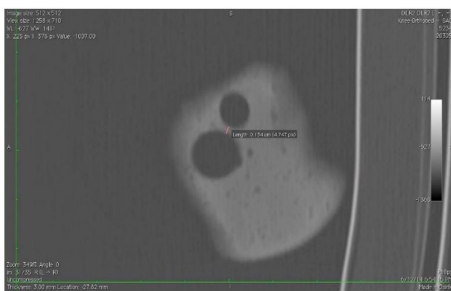
Figure 3: Sagittal CT of outside-in sample with tunnel distance measurement.
