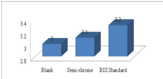
**Figure 10:** Ash content of semi chrome and either indigenous or both improved tanned leathers and BIS standard.
