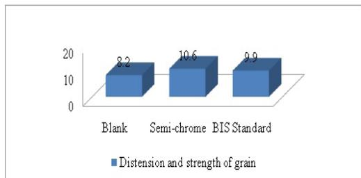
**Figure 6:** Distension and strength of grain of semi chrome and either indigenous or improved tanned leathers and BIS standard.
