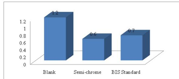
**Figure 9:** Total soluble content of semi chrome and either indigenous or both improved tanned leathers and BIS standard.
