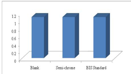
**Figure 1:** Thickness of semi chrome and either indigenous or improved tanned leathers and BIS standard.
