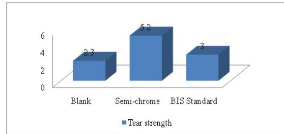
**Figure 3:** Tear strength of semi chrome and either indigenous or both improved tanned leathers and BIS standard.
