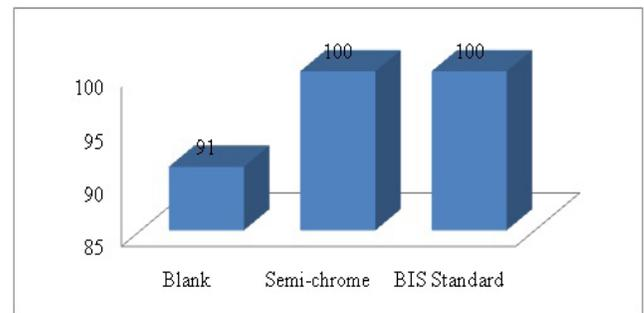
**Figure 7:** Shrinkage temperatures of semi chrome and either indigenous or improved tanned leather and BIS standard.
