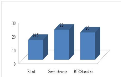
**Figure 2:** Tensile strength of semi chrome and either indigenous or both improved tanned leathers and BIS standard.
