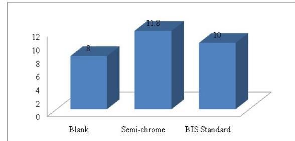
**Figure 4:** Stitch tears strength of semi chrome and either indigenous or improved tanned leather and BIS standard.
