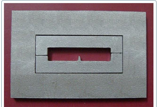
Figure 1: Metal mold for preparation of the bar-shaped composite resin specimens.
