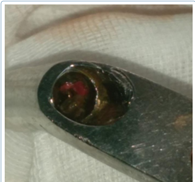
Figure 2: Photograph showing cold welding of barrel plate to Richard screw seen end on.
