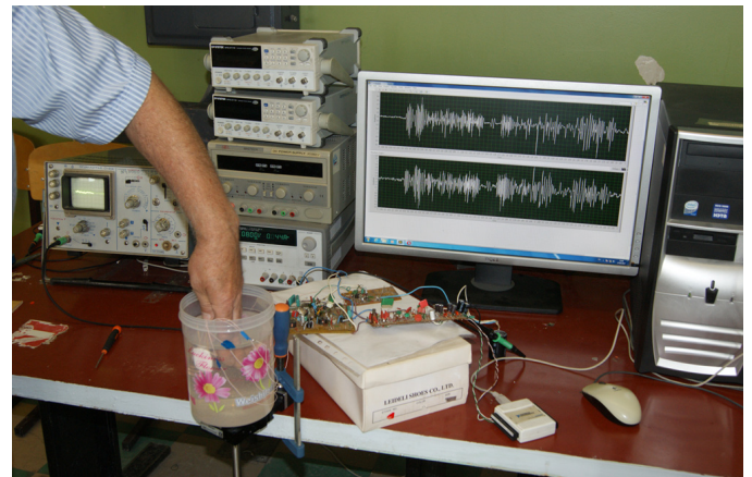
Figure 3: Ultrasonic experimental installation for Tomography of objects in water. The white square from the material absorbing ultrasound on a tank sidewall from the inside contains two piezoceramic elements which carry out function of ultrasonic antennas of a Doppler locator.
