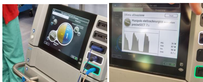
Figure 3: Elettrosurgical monitor unit: energy transmission has been set and there is not spread beyond the point of cauterization.
