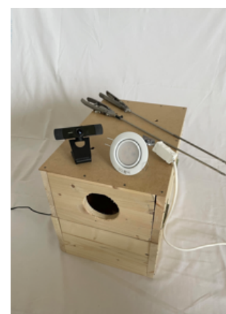
Figure 3: The box with the central hole allowing the insertion of the light source. Above the box: the camera, the light source, and the instrument
