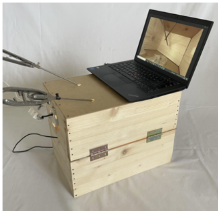
Figure 4: Side view of the 16 liters laparoscopic box
