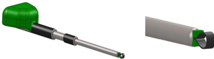
Figure 7: Surgical robotic end effectors and its enlarged tip to measure kinesthetic force feedback for haptic interaction.
