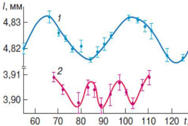
**Figure 4.** Change in Length (Mm) of the Plutonium Specimens with Different Content Of  $^{238}\text{Pu}$  Isotope Against Time (Hours): 1 - 7,3%  $^{238}\text{Pu}$ , 2 - 80%  $^{238}\text{Pu}$ .
