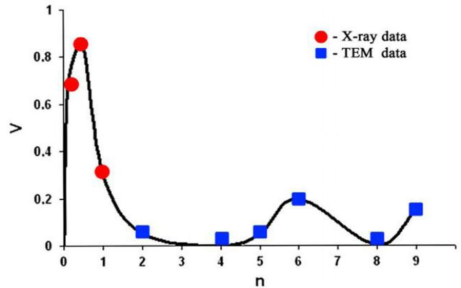
**Figure 5.** Volume Fraction of Crystalline Phase V as a Function of the Number of the Mobile Anvil Rotations N for the Amorphous  $\text{Ti}_{50}\text{Ni}_{25}\text{Cu}_{25}$  Alloy.
