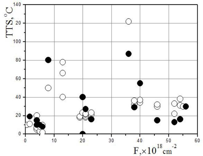
**Figure 3.** Dependence of the TTS on the fast neutron fluence from surveillance data for Spanish nuclear power plants base metal ( $\circ$ ) and welds ( $\bullet$ )
