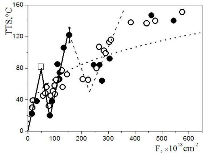
**Figure 6.** Dependence of the Transition Temperature Shift Against Neutron Fluence From Surveillance Data For WWER-440/213 Base Metal and Welds. Where  $\circ$  - flux  $\sim 30 \times 10^{11} \text{cm}^{-2} \text{c}^{-1}$ ,  $\bullet$  - flux  $\sim 4 \times 10^{11} \text{cm}^{-2} \text{c}^{-1}$ ,  $\square$  - flux  $\sim 1,3 \times 10^{11} \text{cm}^{-2} \text{c}^{-1}$ .
