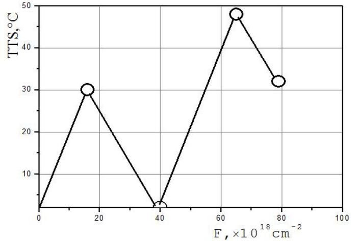
**Figure 2.** Dependence of the Rovno-1 RPV Base Metal TTS on the Fast Neutron Fluence. Neutron Flux  $\sim 6 \times 10^{10} \text{ cm}^{-2} \text{ c}^{-1}$  (Specimens from Upper Containers).
