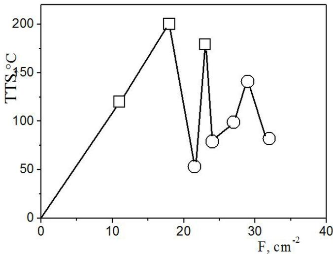
**Figure 1:** Dependence of the Novovoronezh-1 RPV Weld Metal TTS on the Fast Neutron Fluence ( $\square$  - NRC “Kurchatov Institute”,  $\circ$  - IVO Finland). Where  $\circ$  - flux  $\sim 30 \times 10^{11} \text{ cm}^{-2} \text{ c}^{-1}$ ,  $\bullet$  - flux  $\sim 4 \times 10^{11} \text{ cm}^{-2} \text{ c}^{-1}$ ,  $\square$  - flux  $\sim 1,3 \times 10^{11} \text{ cm}^{-2} \text{ c}^{-1}$ .
