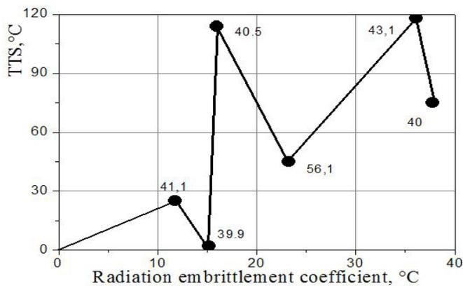
**Figure 7.** Dependence of the Transition Temperature Shift Against Radiation Embrittlement Coefficient (Chemical Factor)  $A_F$  From Surveillance Data for WWER-440/213base Metal and Welds.
