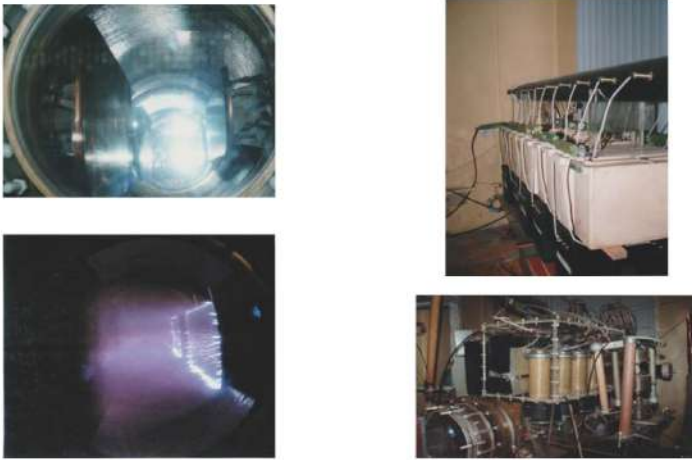
Figure 16: Discharge gap and power source for a non-chain HF laser with P = 407 J.
