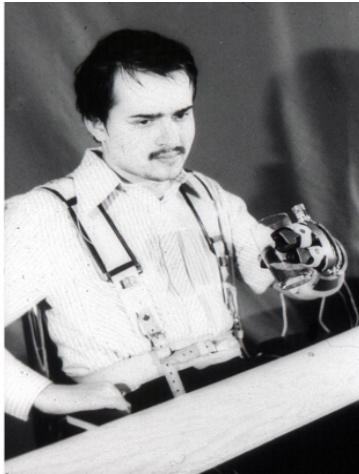
Figure 1: A patient with hybrid orthosis (using nerve stimulation) - enabling the function of the paralyzed tetraplegic hand.
