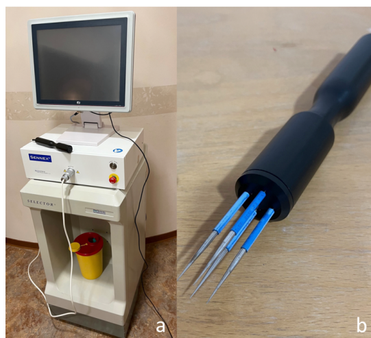
Figure 1: Setup of equipment. a. Sennex® system consisting in monitor (above), generator (beneath) and tray. b. Four prong applicator with electrodes in an unsterile setting.
