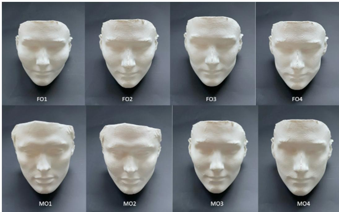
Multiple functions such as 'de-feature,' 'smooth area,' and 'fill area' were used to eliminate borders and make each 3D model look as natural as possible. Each 3D model was saved and exported as an STL file.
