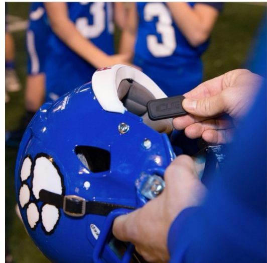
Figure1: Illustration of one American football helmet being fitted with removable and rechargeable accelerometer sensor.
