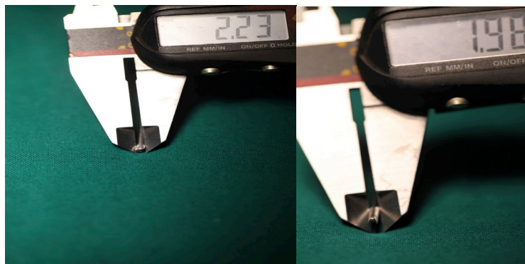
Figure 7: Measurement of outer diameter of ureterscope at distal tip by digital calipers.
