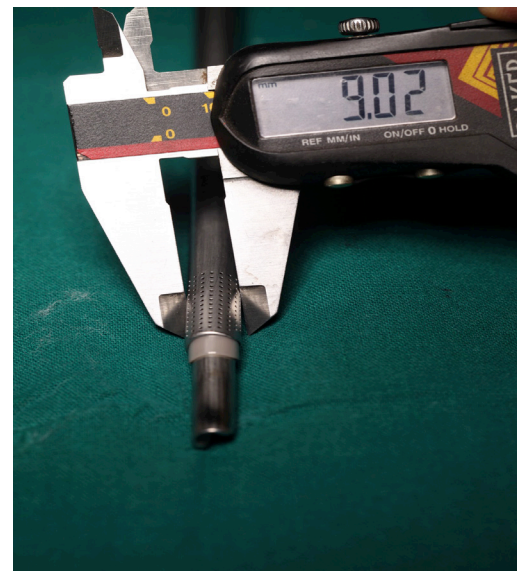
Figure 2: Measurement of outer diameter of TURP sheath at distal shaft by digital calipers. ( 9.02 \times 3.14 = 28.32 ).
