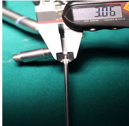
Figure 6: Measurement of outer diameter of ureterscope at proximal shaft by digital calipers.
