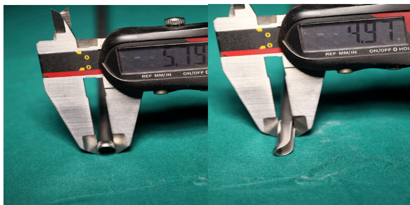
Figure 5: Measurement of outer diameter of cystoscopy sheath at distal shaft by digital calipers.
