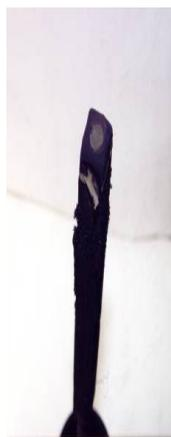
**Figure 2:** Anode which contains platinum and carbon dust.
