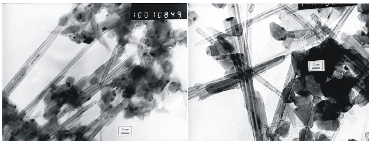
Figure 6: Carbon nanotubes constituting the core of the deposit, obtained by the simultaneous evaporation of a graphite electrode doped with platinum.
