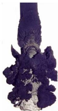
**Figure 3:** Appearance of the platinum-containing deposit on the cathode.
